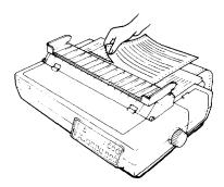
**3.** Press the **TEAR OFF** button again to reverse-feed the paper to its loading position.
